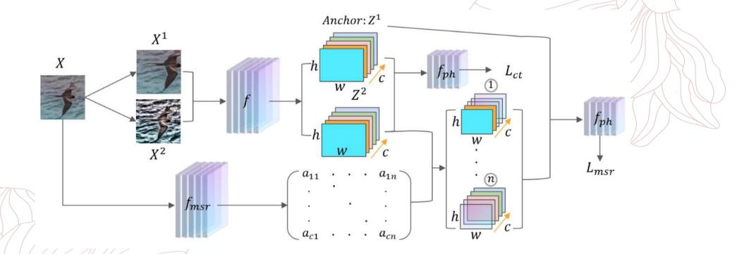
In the first stage, f and  $f_{ph}$  are learned using the two augmented training set  $X_{tr}^{aug}$ , and the semantically relevant weight matrix  $A_s$ . In the second stage,  $f_{msr}$  is updated by computing its gradients with respect to the contrastive loss.
